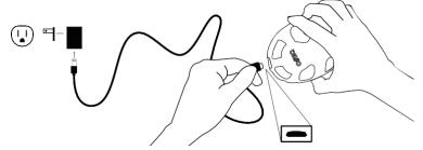
Plug the micro-USB end of the cable into the charging port located on the end of Oska Pulse.
