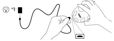
Plug the micro-USB end of the cable into the charging port located on the end of Oska Pulse.
